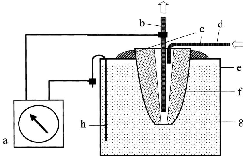
**Figure 1** Experimental setup of intracanal aspiration technique (IAT). (a) Root ZX. (b) Aspiration needle. (c) Self-curing resin. (d) Washing needle. (e) Plastic case. (f) Tooth. (g) Coloured agar. (h) Neutral electrode. The irrigant injected from the tip of the washing needle (d) was ejected by the tip of the aspiration needle (b).
